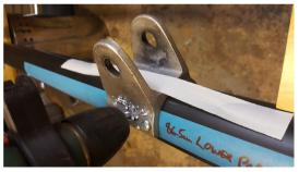
Drill holes for the the goose neck and other fittings as per the Comet dinghy instructions and using the marks made on the masking tape as a guide.
