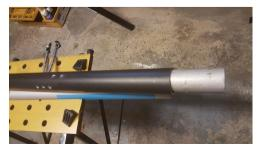
The old holes are then filled with JB Weld and the excess scraped off after a couple of hours (whilst it is still tacky) and the surface cleaned. Note that the JB Weld seems to sink a little but that's fine. If I was a total perfectionist I would fill, sand an paint but as the holes are below deck height the aesthetics don't worry me.
