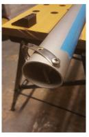
Trial fit first to make sure everything lines up and note that the inboard end of the lacing eye and the two outhaul block rivets are the short ones as they don't go into the plastic of the boom plug.
