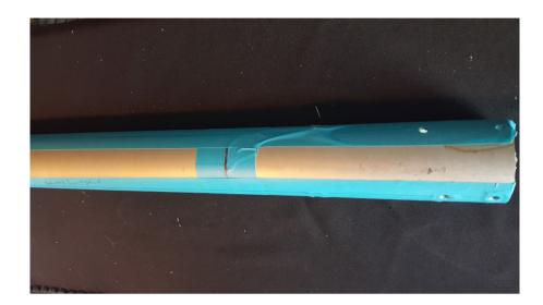
Now repeat the method used to align the lower mast fittings, running tape along the boom and then making a straight pencil line along the old lacing eye and out haul pulley fitting rivet holes.
