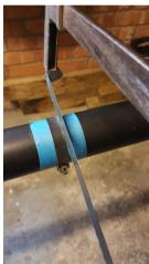
Once everything is measured and marked you can cut the spar at the 570mm mark, working slowly and checking alignment to get a clean cut across, then clean up the burrs.
