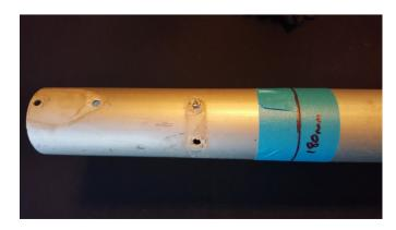
Measure and mark with pencil in three places around the circumference of the boom, then line up a length of masking tape against the pencil marks, and then run a second line of tape next to the first.
