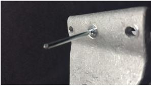
Use the correct rivet length for each and careful with that countersink middle rivet on the PORT side. Make sure the cleat faces the bow and can sit flush before riveting it with the two remaining countersink rivets and use the nuts supplied as spacers to make sure the gun doesn't catch the cleat.
