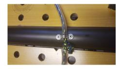
Make good the old rivet holes. You can just fill them up with sealant but I wanted a maintenance free solution, so I took the sliced off bit of boom, cut a slot in it, then crushed it into a smaller tube that just fits inside the lower mast. I used Araldite 2 pack adhesive to secure this inner tube.
