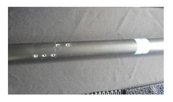
Measure, mark and cut 570mm off the bottom of the lower mast. I measured three points around the mast, then marked them in pencil, then measured the pencil marks to check.
