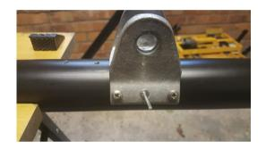
I used a couple of 5mm screws to make sure the fitting didn't move whilst riveting. They are not a tight fit as I didn't want to cut threads into the faces of the holes.
