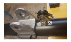
The outhaul pulley and kicker lacing eye are fitted using the short standard rivets and carefully aligned with the centre of the goose neck. I drew a centreline on mine to get it dead centre.
